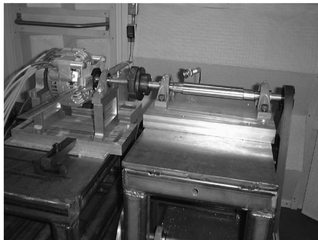
Fig. 3. Test fixture for torque ripple measurement. Extended shaft machine is supported in two additional external bearings. Rotational constraint is provided by a leaf spring restrained by a force transducer.
